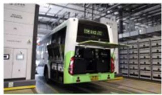
E-bus with swappable batteries in China
